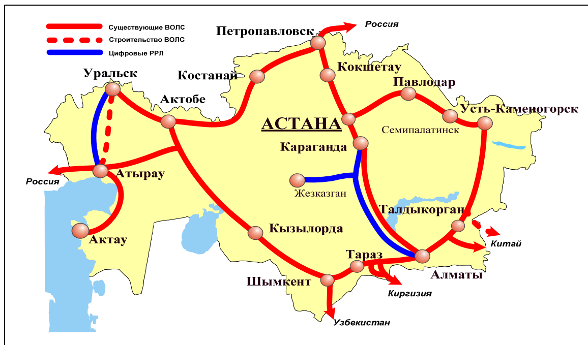
Figure 4: Scheme of fiber-optic backbone of Kazakhstan
